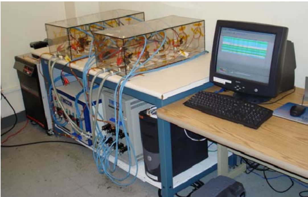
Figure 38. MACCOR battery test system.
