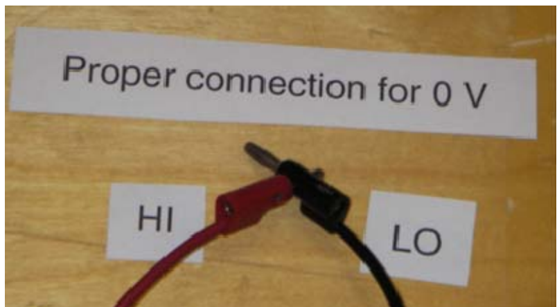
Figure 41. Proper connection for 0 V.
