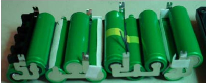
Figure 36. Graphite cells removed from Sony BP-GL95 battery pack.
