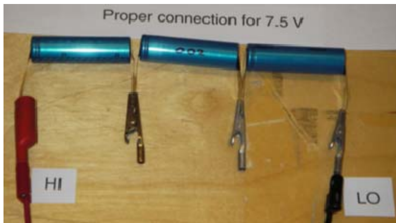
Figure 44. Proper connection for 7.5 V.
