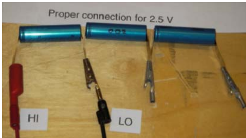
Figure 42. Proper connection for 2.5V.
