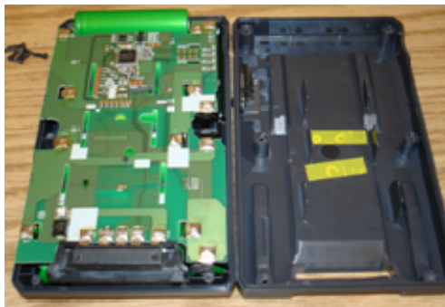
Figure 35. Sony BP-GL95 with cover removed.
