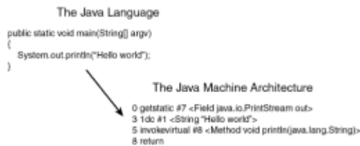
Figure 1.1: Java defines a low-level architecture and instruction set closely aligned with the high-level language.
