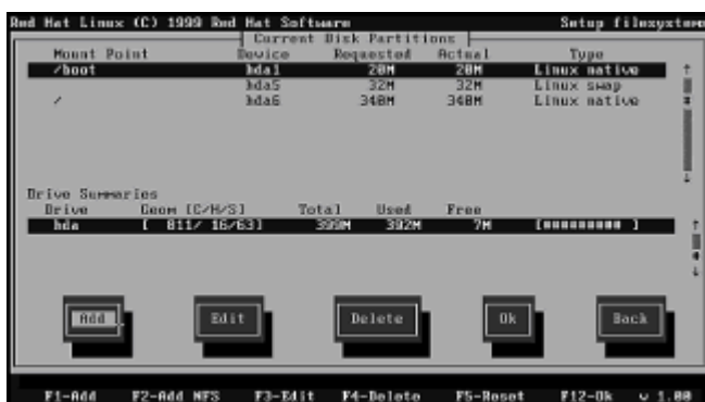
Figure 6.7: New drive configuration, after deleting the Windows partition and creating three new partitions.
