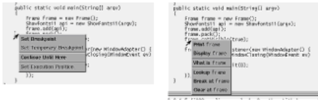
Figure 40.2: Pop-up menus from the right mouse button allow you to control breakpoints and examine variables.
