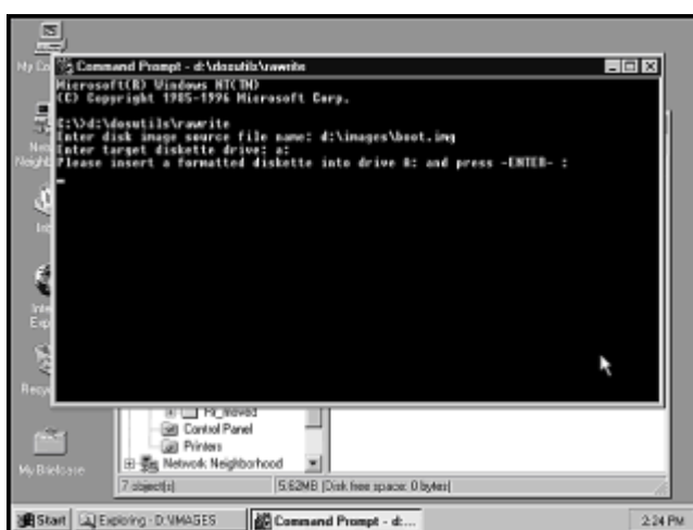
Figure 6.1: Running the RAWRITE.EXE utility to create Linux boot disks from a Microsoft Windows environment.
