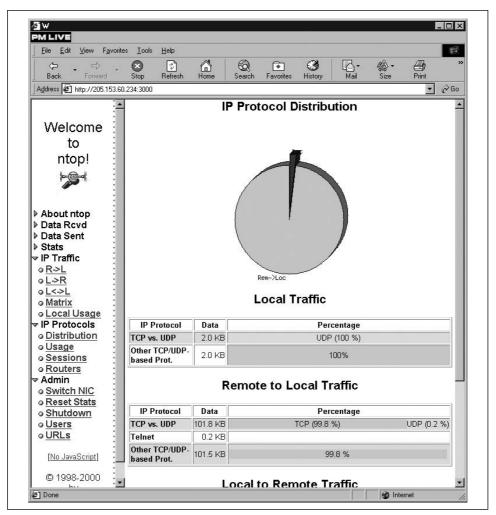
Figure 8-5. Measuring local and remote traffic
