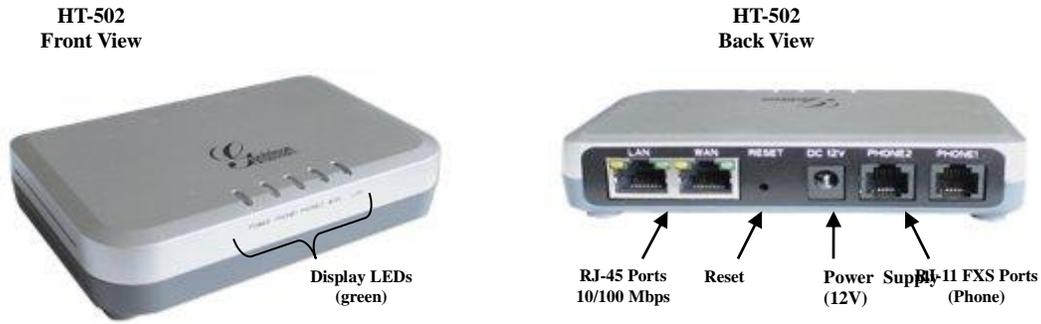
**FIGURE 1: CONNECTING THE HT502**
