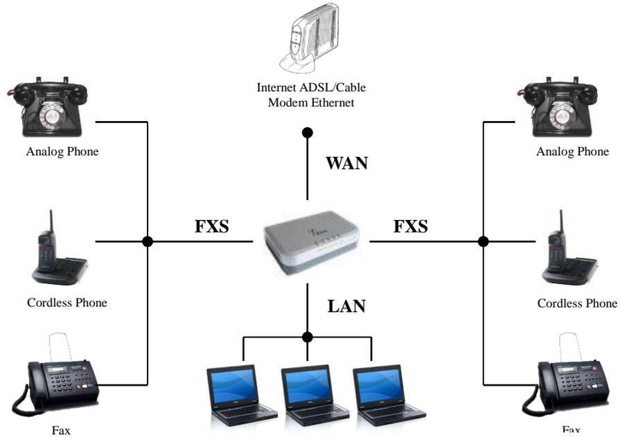
**FIGURE 2: HT502 CONNECTION DIAGRAM**
