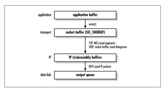
Here is just a short trip through the network layer to explain what happens where. Your application can send any size data to the transport layer, which is either UDP or TCP. The socket buffers are implemented on the transport layer. Depending on your choice of transport protocol, different actions are taken on this level (see Figure C.4Figure C.4).
