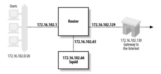
The Extreme switch can intercept HTTP connections only for packets that it routes between subnets. In other words, if you use the Extreme switch in layer two mode (with a single VLAN), you can't divert traffic to Squid. To make HTTP interception work, you must configure separate VLANs for users, Squid, and the Internet:
