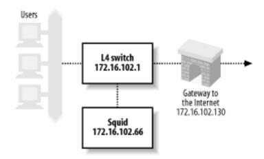
Clients are connected to port 1, the connection to the Internet is via port 2, and Squid is on port 3. The following lines are the relevant output of a /cfg/dump command on the switch. You don't necessarily need to type all of these lines. Furthermore, some of the commands may have changed for newer versions of Alteon's software. Note that Alteon calls this feature Web Cache Redirection (WCR). Here's the process, step by step:
