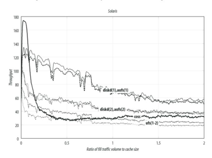
Solaris also supports *coss*, but at nowhere near the rates for Linux and FreeBSD. For some unknown reason, *coss* on Solaris is limited to 32 transactions per second.
