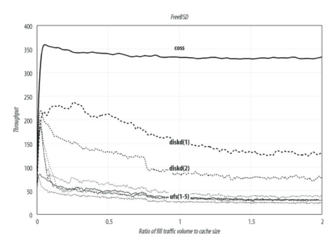
Enabling the async, noatime, and  $softupdate^{[3]}$  options boosts the standard ufs performance from 24 to 38 transactions per second. However, using one of the other storage schemes increases the sustainable throughput even more.
