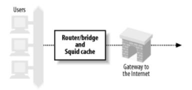
This configuration essentially skips the first three steps shown in <u>Section 9.1</u>. The Squid host already receives the HTTP connection packets because it is the router for your network. If you are taking this approach, feel free to skip ahead to <u>Section 9.4</u>.
