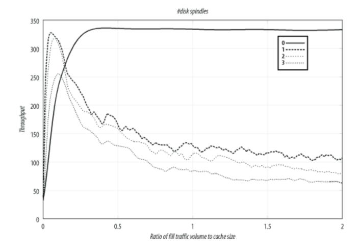
The primary purpose of these tests is to show that Squid's performance doesn't increase in proportion to the number of disk drives. Excluding other factors, you may be able to get better performance from three systems with one disk drive each, rather than a single system with three drives.
