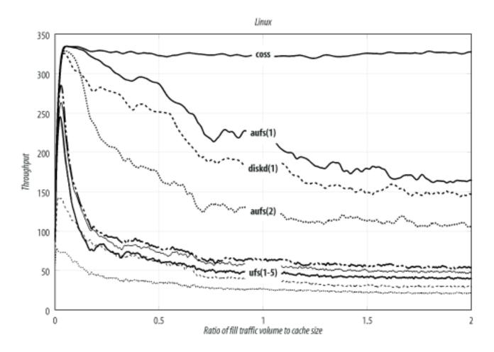
Note that the noatime option gives a significant boost in performance to *aufs*. The throughput jumps from 110 to 168 transactions per second with the addition of this *mount* option. Linux also has an *async* option, but it is enabled by default. I did not run any tests with *async* disabled.
