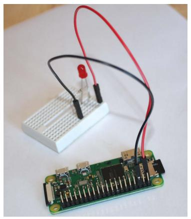
FIGURE 2.2: Male header with female-to-male leads
