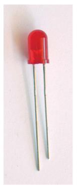
**FIGURE 2.5:** An LED. The long lead is the positive side.
