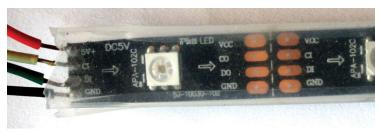
FIGURE 4.3: The arrows show the direction of the DotStar string.
