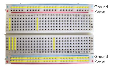
FIGURE 2.6: Solderless breadboard. The yellow indicates which holes are connected.
