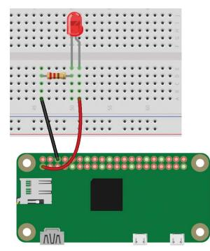
FIGURE 2.8: LED wired to 3.3V power
