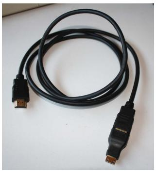
FIGURE 1.3: An HDMI cable with a mini-HDMI adapter
