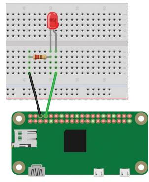
FIGURE 2.9: An LED hooked up to GPIO 14
