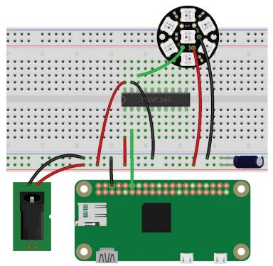
**FIGURE 4.11:** Wiring a NeoPixel light string with the 74LVC245 Octal Bus Transceiver with 3-State Outputs
