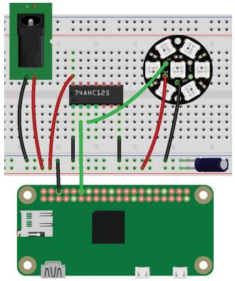
**FIGURE 4.12:** Wiring a NeoPixel light string with the 74AHCT125 Quad Buffer/Line Driver, 3-state
