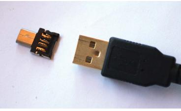
FIGURE 1.6: A USB On-the-Go (OTG) adapter
