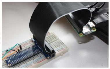
FIGURE 2.4: A GPIO extension, with ribbon cable and a breadboard
