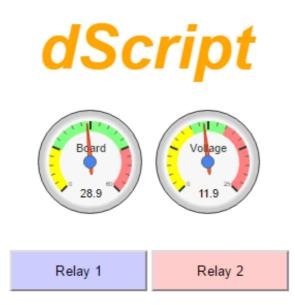
The left gauge measures the board temperature using the on-board temperature sensor. The right gauge is the boards supply voltage.
